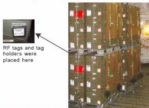
Figure 8. RF Tag Placement During Transport to the USS Harry S. Truman: Thirty-two RF tags were placed on the munitions pallets at CAAA, IN and shipped by commercial ground to the Norfolk Naval Station, VA.
