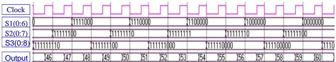
Figure 44. RSNS-to-Binary Waveform Outputs for Dynamic Range Values 48:60
