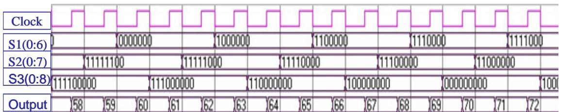
Figure 45. RSNS-to-Binary Waveform Outputs for Dynamic Range Values 60:72
