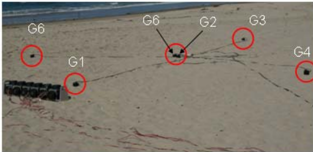
Figure 29. Geophones Placed Both in Line and in Angular Positions (5 Sep 2005)
