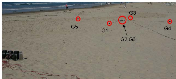
Figure 30. Geophones Layout with G1 Placed at 48 Feet from the Source (5 Sep 2005)
