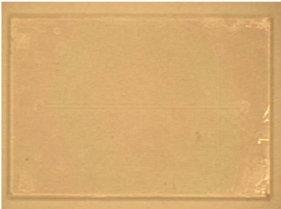
Figure 64. Photograph of a glass substrate with etched channels which has a thin layer of the new thermoplastic adhesive covering the top surface.
