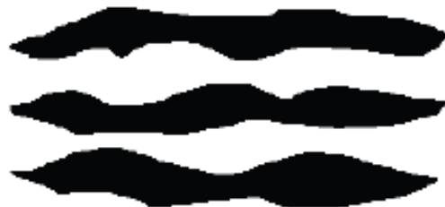
Figure 51. Concept of phenolic conforming to a "rough" membrane topography and planarizing for multiple stacked layers.
