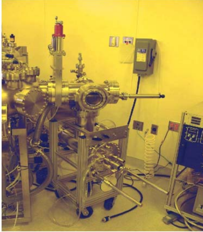
Figure 47. Evaporator system developed for fabricating the membranes.
