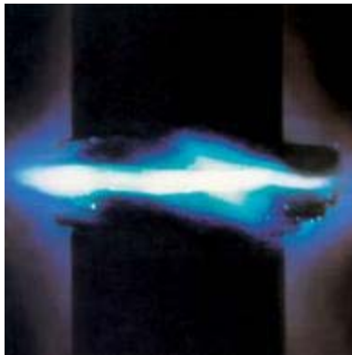
Figure 3-Vacuum Arc between Two Electrodes [5]
