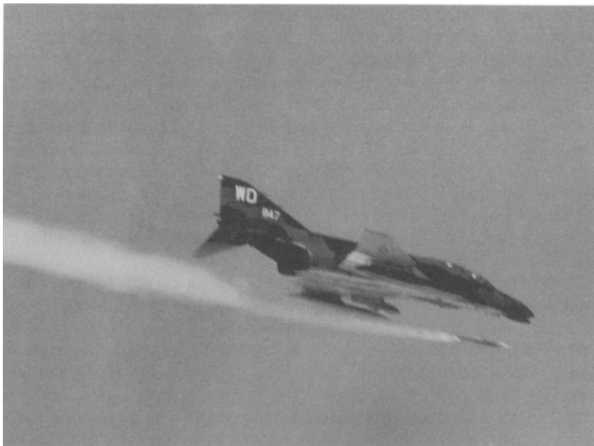
F-4C aircraft were specially equipped to counter enemy radar-controlled ground defenses.
