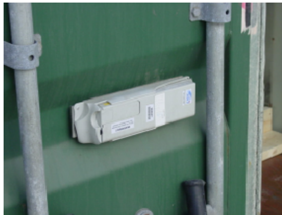
Figure 17. RFID Tag used during OIF3 to track containerized cargo (Courtesy of Henry Cook)
