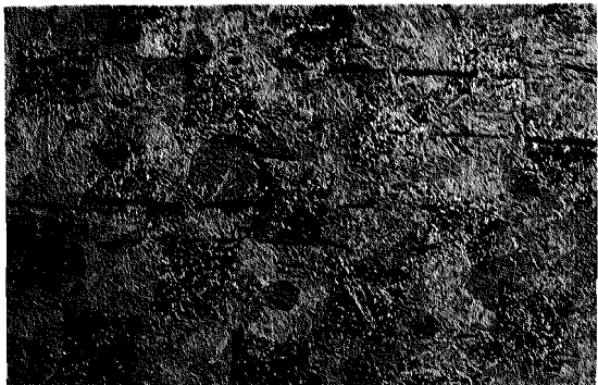
X100 -C- PICRAL SURFACE OF PROJECTILE AT BOURRELET- STREAKS OF FINE ELONGATED INCLUSIONS.
