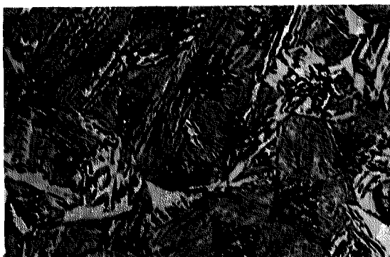
X1000 -F- PICRAL CENTER OF PROJECTILE AT BOURRELET- SAME LOCATION AS E. SOME MARTENSITE WITH LARGE AMOUNT OF BAINITE AND FERRITE.
