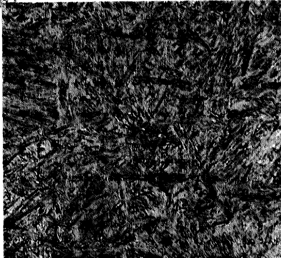
X1000 -B- PICRAL FORWARD CORNER OF PROJECTILE NOSE-- SAME AREA AS A. MARTENSITIC STRUCTURE.
