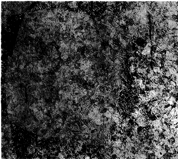
X100 -C- PICRAL FORWARD OF EXPLOSIVE CAVITY— FINE SEGREGATIONS OF INCLUSIONS, SOME BANDING.
