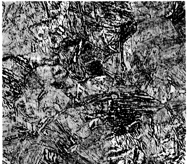
X1000 -D- PICRAL FORWARD OF EXPLOSIVE CAVITY— SAME AREA AS C. MARTENSITE AND MODERATE AMOUNT OF BAINITE.
