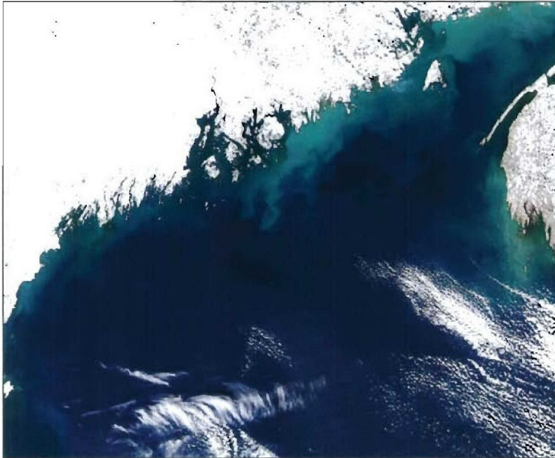
Figure 8. Example 250 m resolution MODIS Aqua “true-colour” products of the Gulf of Maine / Southwest Nova Scotia showing surface turbidity/colour patterns, vapour trails, internal wave patterns and bottom bathymetric features.
