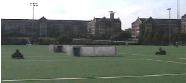
b) Communications is broken and the robots begin the execution of their recovery behaviors. The robot on the left executes Retrotraverse , the robot on the right executes Move-To-Nearest-Neighbor .
