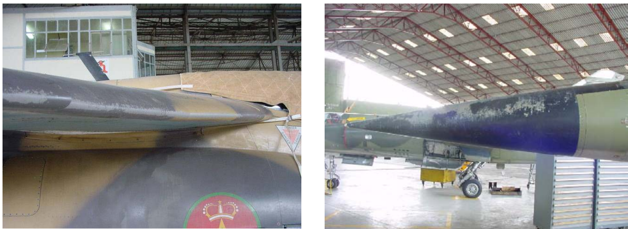
Fig. 8 AlphaJet wing leading edge erosion (left) and Mirage F1 nose cone erosion (right)
