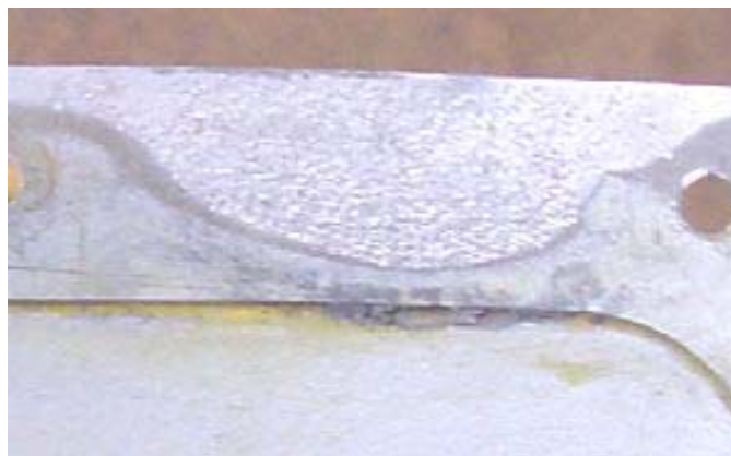
Fig. 5 Fretting of contact area between Alphajet fuselage and tail cone
