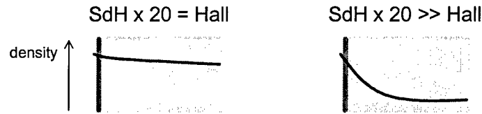
Figure 12: The inferred density profile through the multiple QW region (left) early and (right) late in the MBE growth run.
