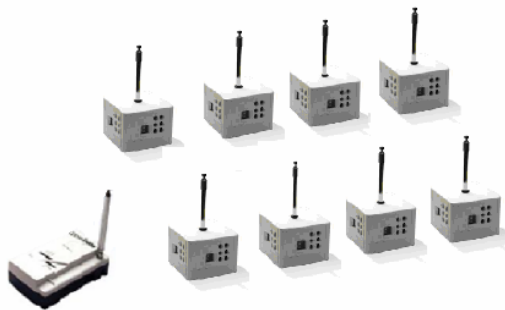
Figure 3. Mote Security System MSP 410CA
