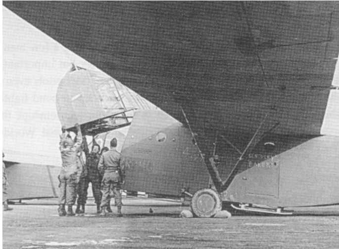
Down easy: the hinged cockpit of a Waco is lowered into place. Visible to the right of the glider's wheel are its wooden skids. (Courtesy Smithsonian Institution)
