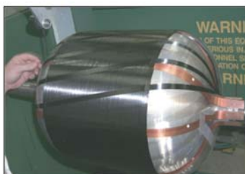
Figure 3: Piezoelectric sensor based SMART Layer ® network integration
