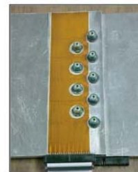
Figure 3: Piezoelectric sensor based SMART Layer ® network integration
