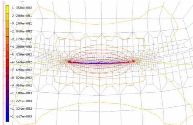
Fig. 8: Closed-up of the radial stresses between Si<sub>3</sub>N<sub>4</sub> and AISI 4140
