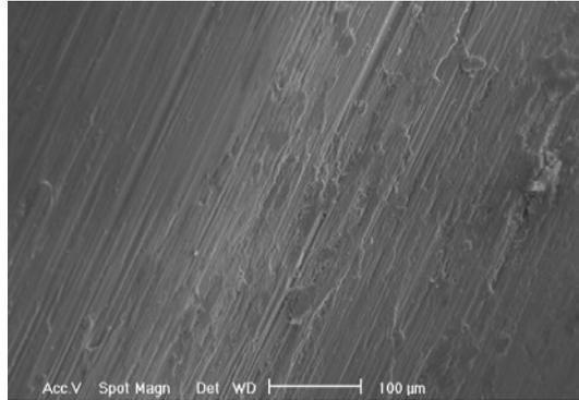
Fig. 4: SEM micrographs showing Ti-6Al-4V surface wear
