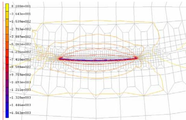
Fig. 9: Closed-up of the radial stresses between Si<sub>3</sub>N<sub>4</sub> and Ti-6Al-4V
