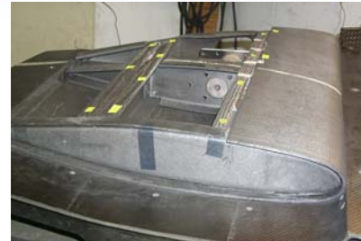
Sharp leading edge, T > 3600^{\circ}\text{F}
