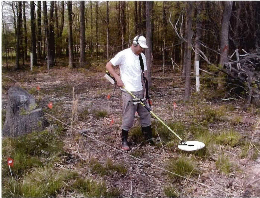
Figure 1. GEM-3 EMI/Hand Held demonstrator's system.
