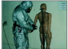
who conducted standard law enforcement activities that might be performed on the incident scene. The study tested four chemical protective ensembles, a mechanic's asbestos overalls and the standard MSP duty uniform. Testing was conducted in the SBCCOM MIST test facility.
