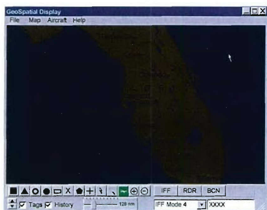
Figure 16. Situation Display with permanent primary menu bar (top) and toolbars and hot buttons allocated to a fixed location
