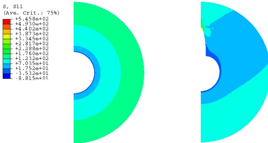
Figure 3: Stress Fields in Uncracked and Cracked Thermal Analog Motors (Case Not Shown)
