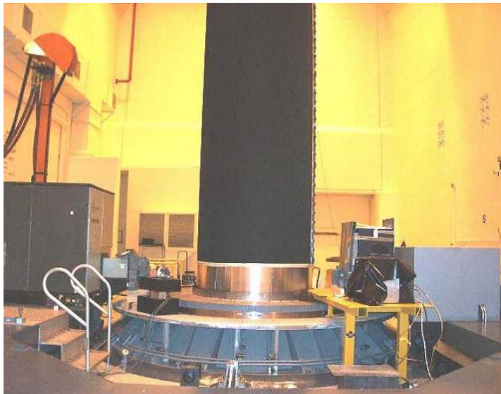
Hill AFB High Resolution 3D Computed Tomography (HR3DCT) Facility Inspecting Large Steel Case Boost Motor
