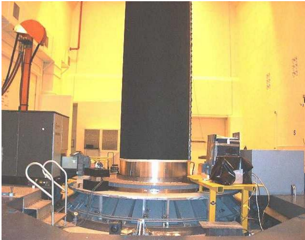
Figure 2: Hill AFB High Resolution 3D Computed Tomography (HR3DCT) Facility Inspecting Large Steel Case Boost Motor
