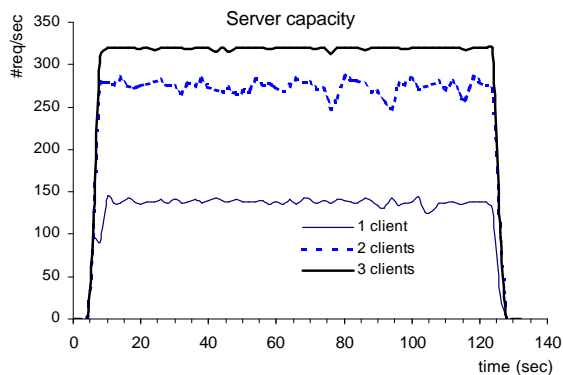
Figure 7: Three client machines saturate the web server with 320 requests per second.
