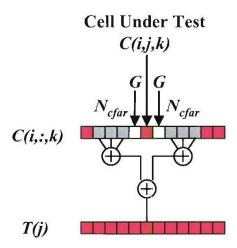
Figure 1. Sliding window in CFAR detection. The example shows the number of guard cells G=1 and the number of cells used in computing the estimate  $N_{cfar}=3$ .
