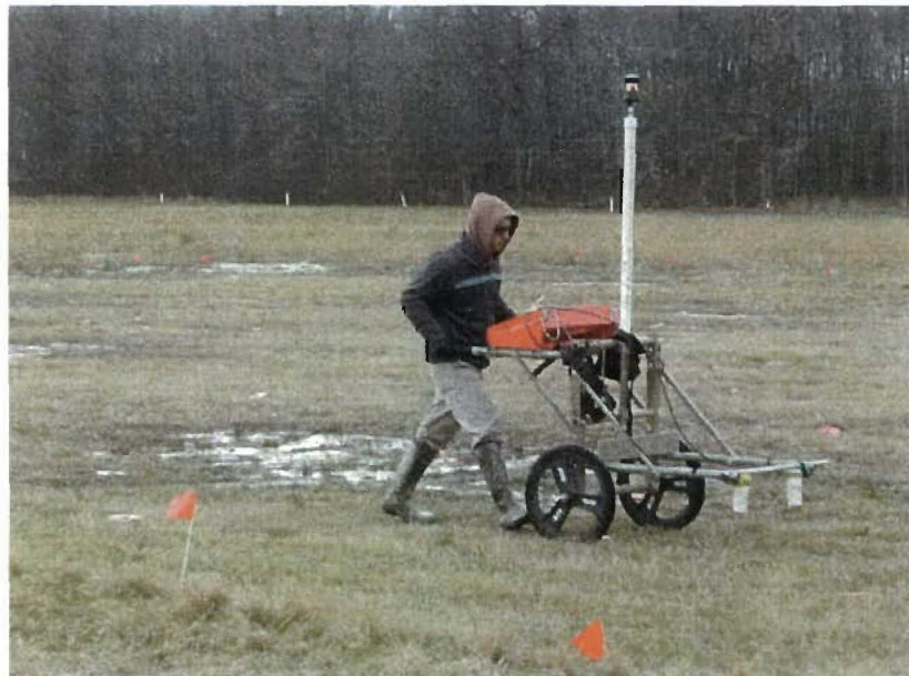
Figure 1. Shaw UXO Mapper (dual sensor G858 magnetometer).
