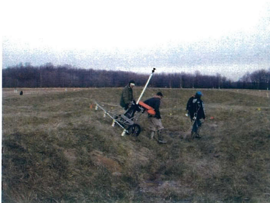
Figure 1. Shaw UXO mapper (G858 magnetometer array configuration).
