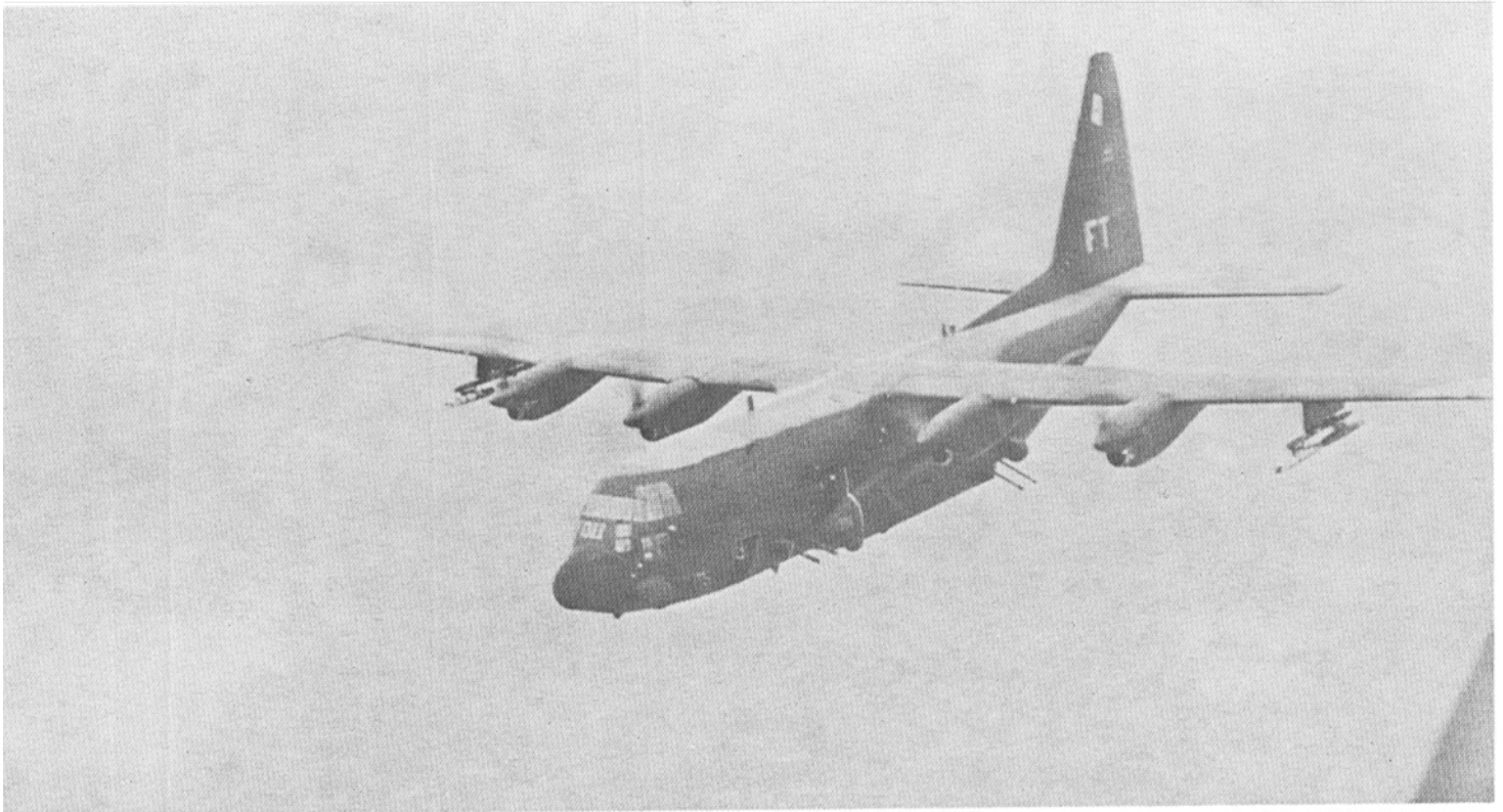
AC-130 "Spectre" Gunship—Note 20mm and 40 mm guns protruding from the side.
