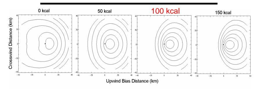
Monte Carlo analysis of UV plume as 2-step mechanism sensitive to ACTIVATION ENERGY in the final step.
