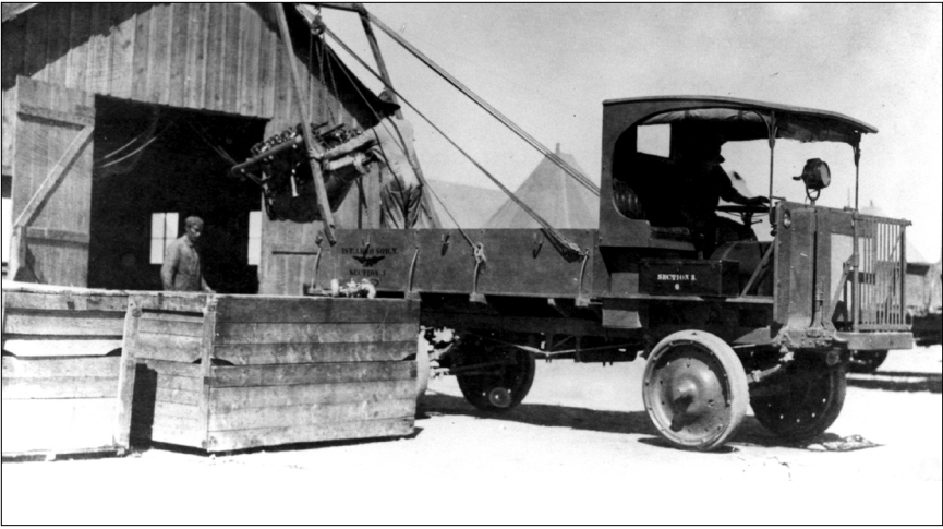
A derrick mounted on the rear of a Jeffery truck turned it into a crane capable of moving an engine to and from the machine shop at Columbus, New Mexico.
