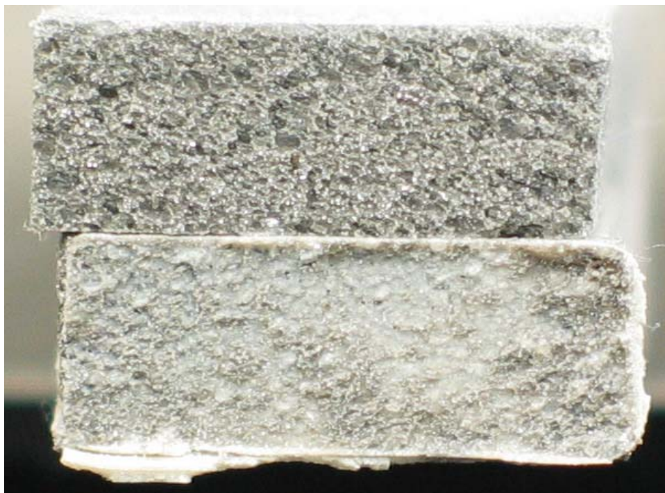
Fig.2. Fracture Surface (Displacement Rate = 2.54 cm/min).
