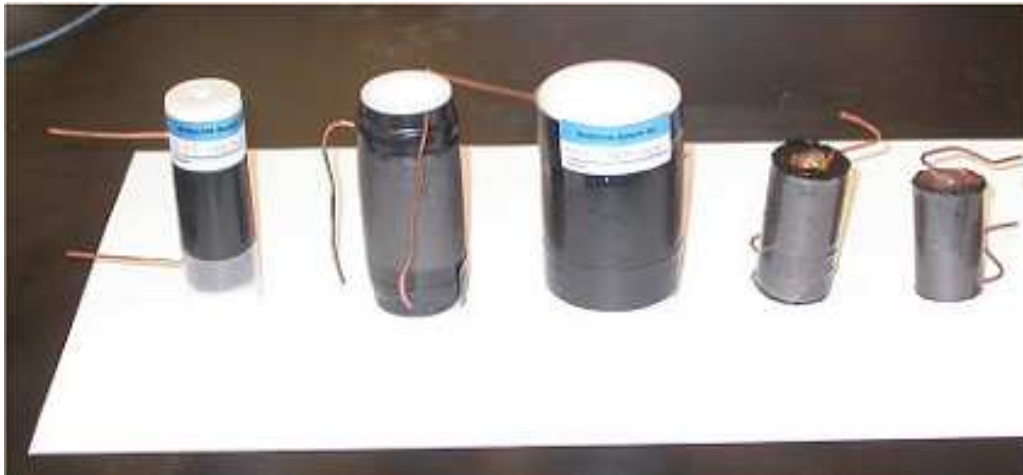
Figure 7. Rolled dielectric actuators fabricated from silicone and polyurethane dielectric layers.
