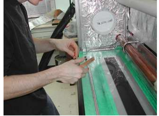
Figure 5. Apparatus for fabrication of rolled dielectric actuators.
