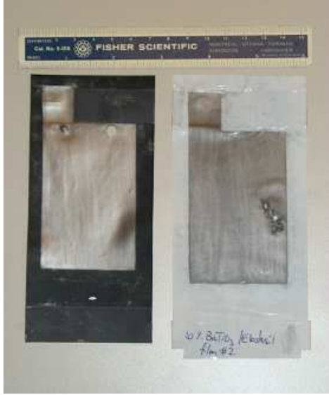
Figure 4. Photograph of film actuators filled with high dielectric constant fillers. Left: Poly(copper phthalocyanine)/ EVA composite film. Right: Barium titanate/ elastosil film.
