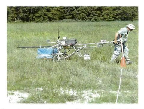
Figure 1. Demonstrator's system, Simultaneous Magnetometry and Pulsed EM/man-portable.
