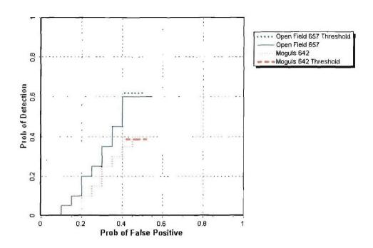
Figure 9. Combined Sensor/man-portable  $P_d^{disc}$  versus the respective  $P_{fp}$  for ordnance larger than 20 mm.
