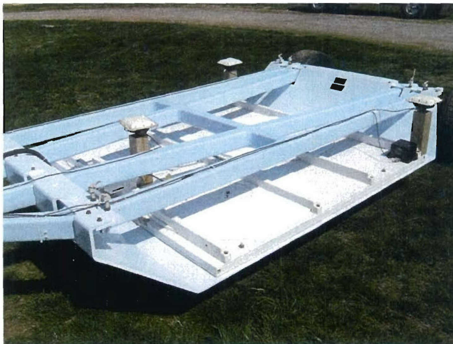
Figure 1. Demonstrator's system (MTADS GEM array on tow platform showing three sensors, three GPS antennae, and the IMU).
