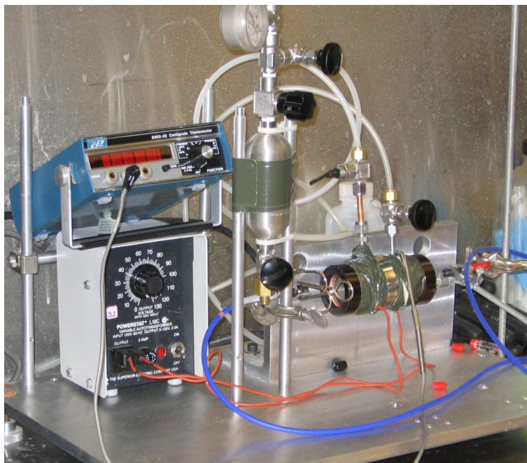
Figure 1: Gas cell connected in-line with the UV-vis spectrometer. The blue cables are the optic fibres connected to the Ocean Optics spectrometer. The cell is wrapped in heating tape for temperature control although this feature was not utilized in this work. Two Teflon gas-handling lines exit out of the top of the cell: one equipped with a toggle valve and the other with a needle valve. The gas cylinder attached to the aluminum post was not used for these experiments. For clarity, the gas bulb and water bath have been removed so that the cell can be seen.
