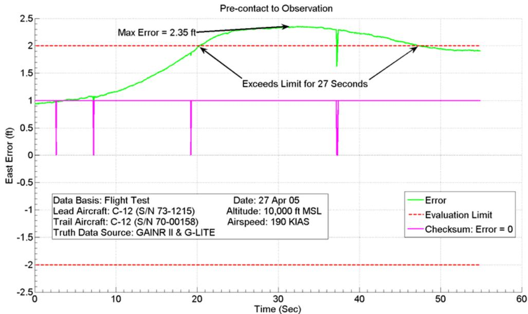
**Figure 2: East Error During Pre-contact → Observation Maneuver**
