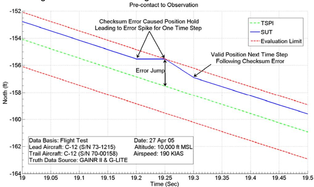
**Figure 4: Position Error Caused by Checksum Error**
