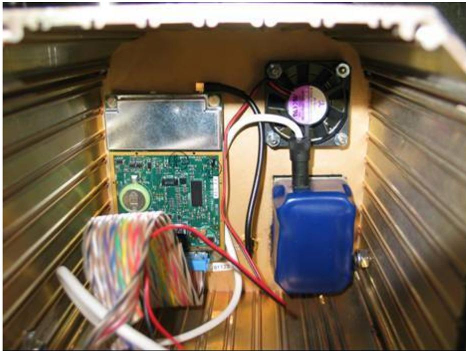
**Javad GPS Receiver Card (left) and MEMS IMU (lower right)
