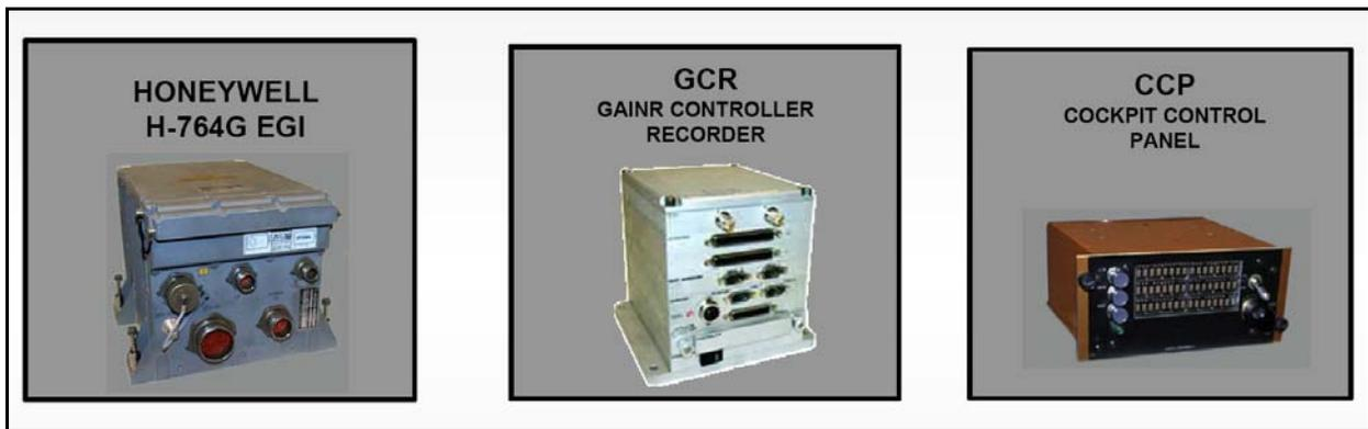
**Figure A-3: Components of the GPS Aided Inertial Reference System**
