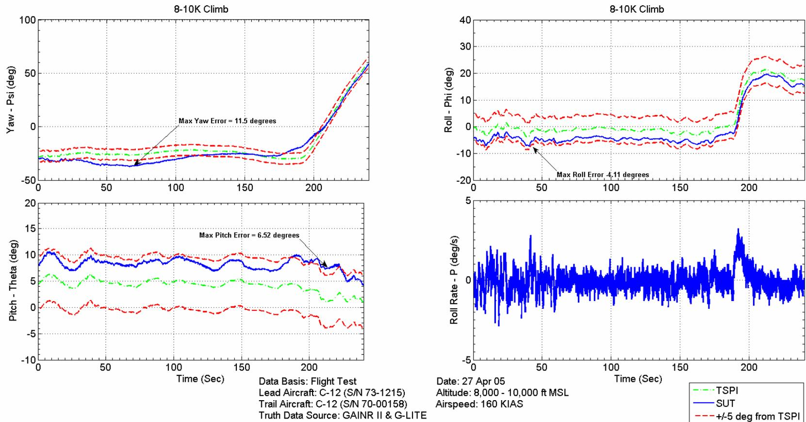
**Figure D-18: MEMS IMU Error during Climb from 8,000 PA to 10,000 PA**
