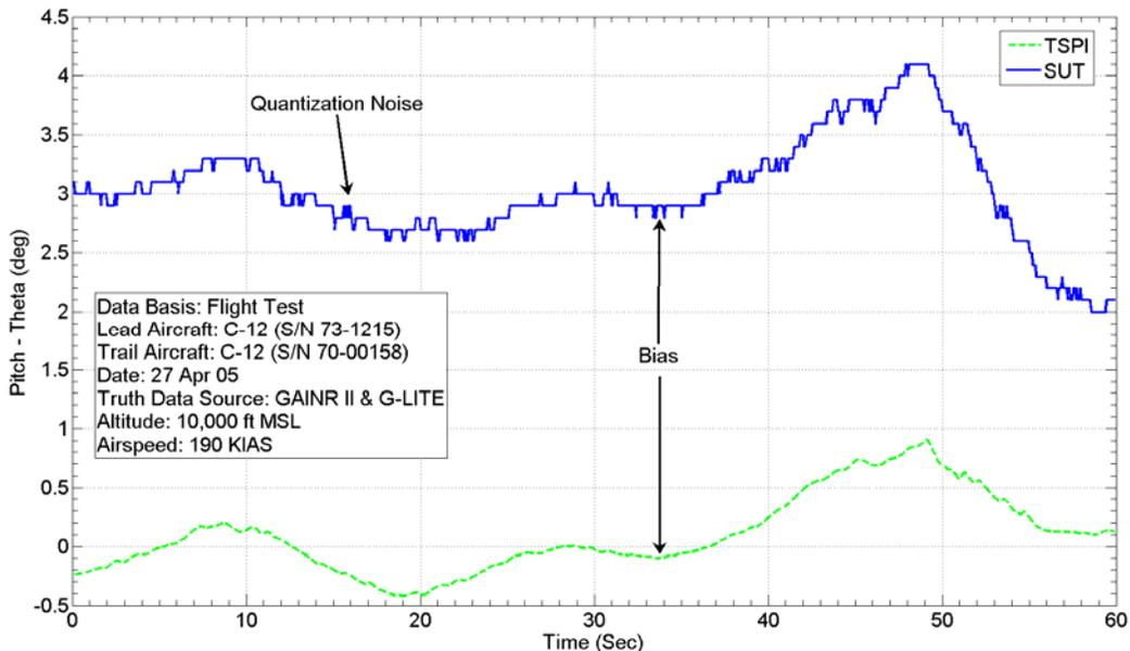
**Figure 7: Pitch Output Noise Due to 0.1 Degree Quantization**
