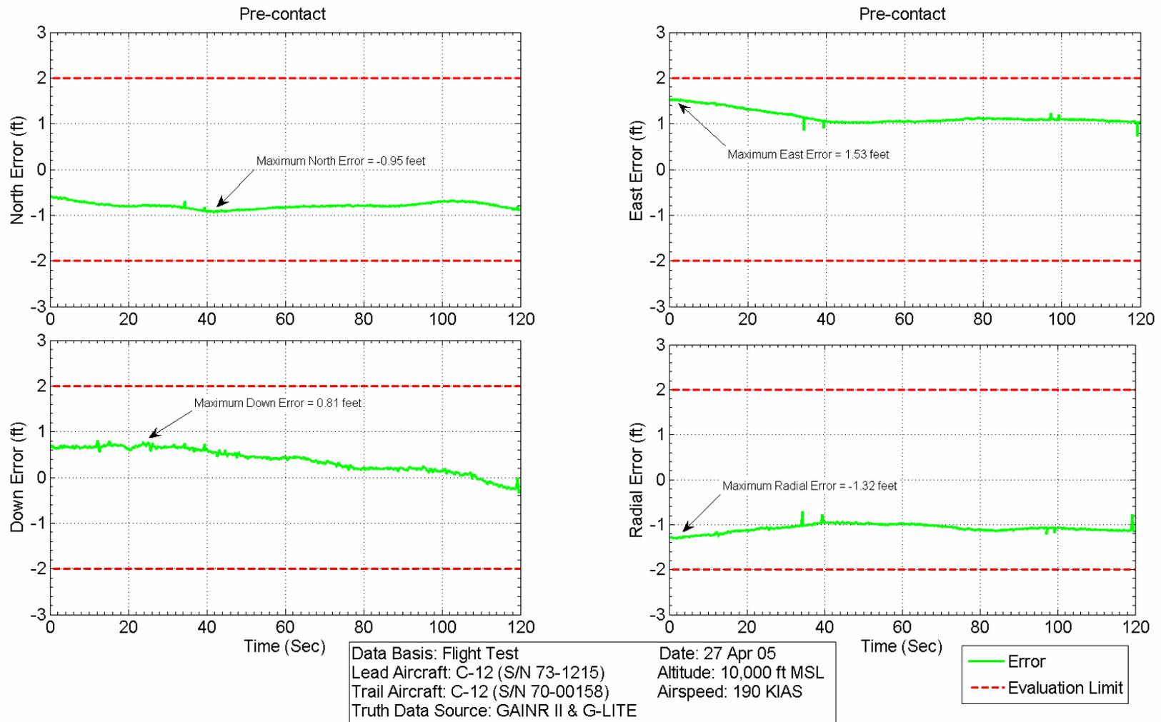
**Figure D-6: Relative GPS Position Error in the Pre-contact Position**
