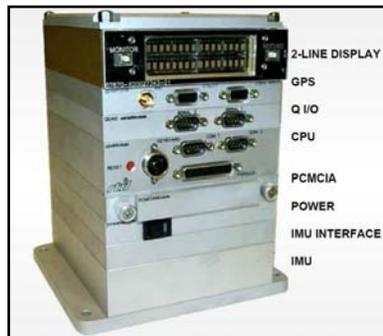
**Figure A-4: GPS Aided Inertial Reference System – Lite**
