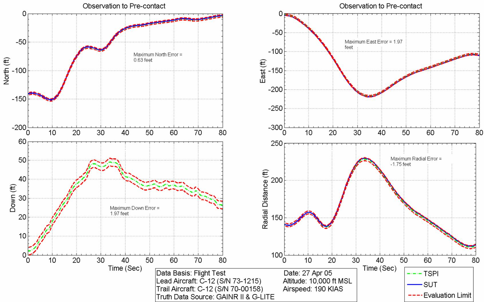
**Figure D-9: Relative GPS Position Comparison between SUT and truth source during the Observation Position to Pre-contact Position transition**
