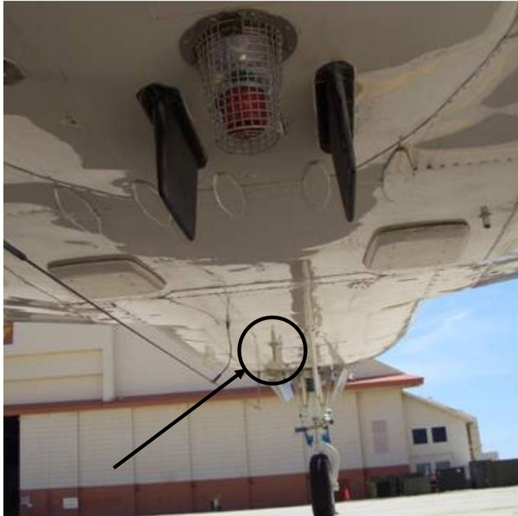
**Figure A-2: C-12C Tail # 73-1215 Datalink Antenna**
