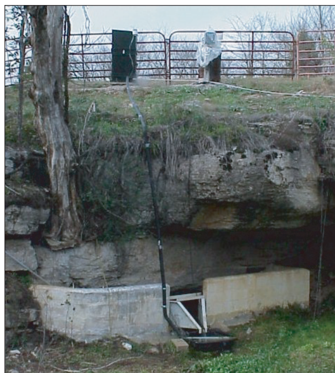
Figure 3. Water-quality monitoring and volatile organic compound sampling equipment at Wilson Spring.
