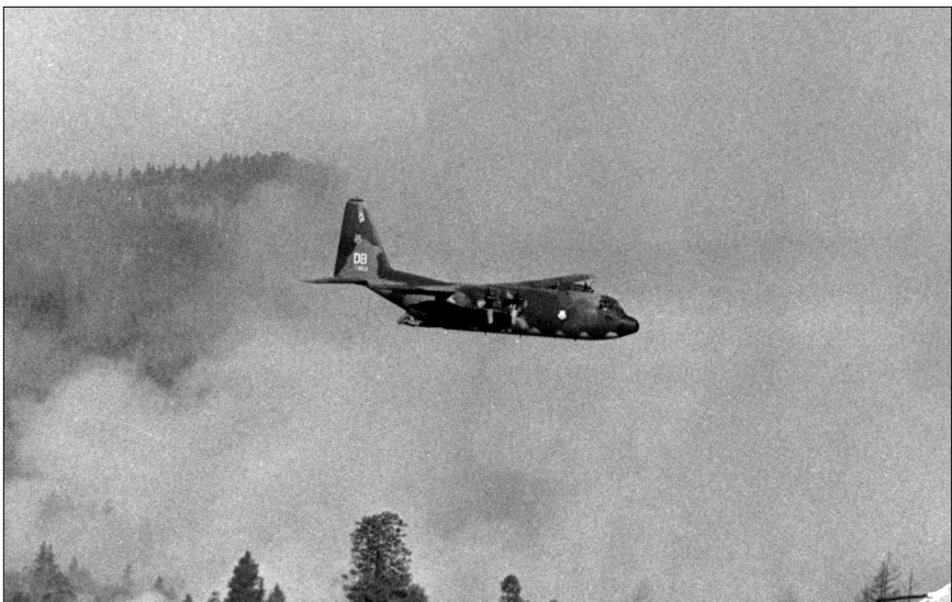
A C-130 equipped with the Modular Airborne Fire-Fighting System flies into a fire zone in northern California to drop fire-retardant chemicals to control the blazes. (NARA photo.)
