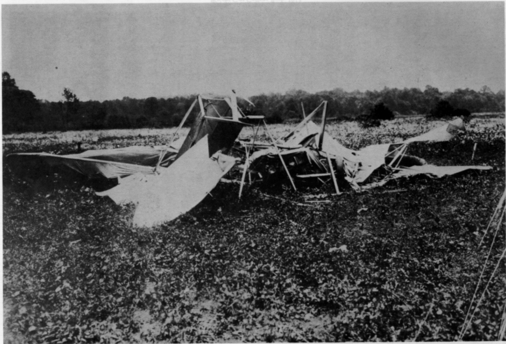
Wreck of Wright C, Signal Corps No. 10, in which Welsh and Hazlehurst were killed at College Park
