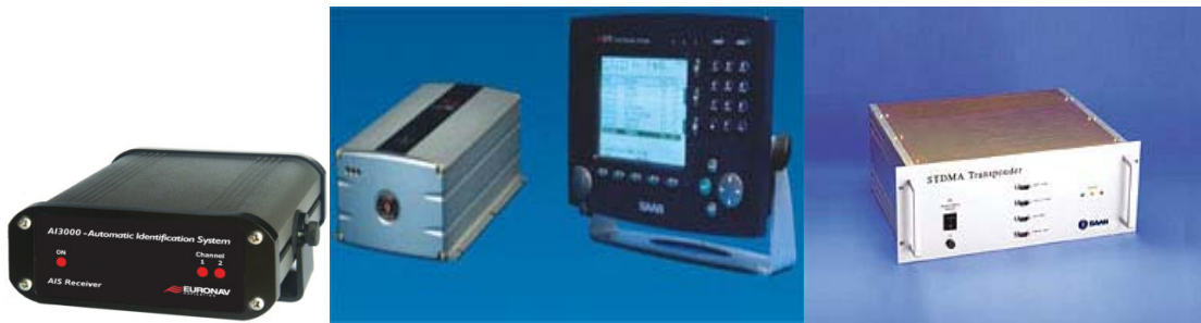
Figure 5. (a) Receive-only unit (b) Mobile AIS transponder (c) Base-station transponder. A mobile AIS transponder need not move around, nor need a base-station be immobile.
