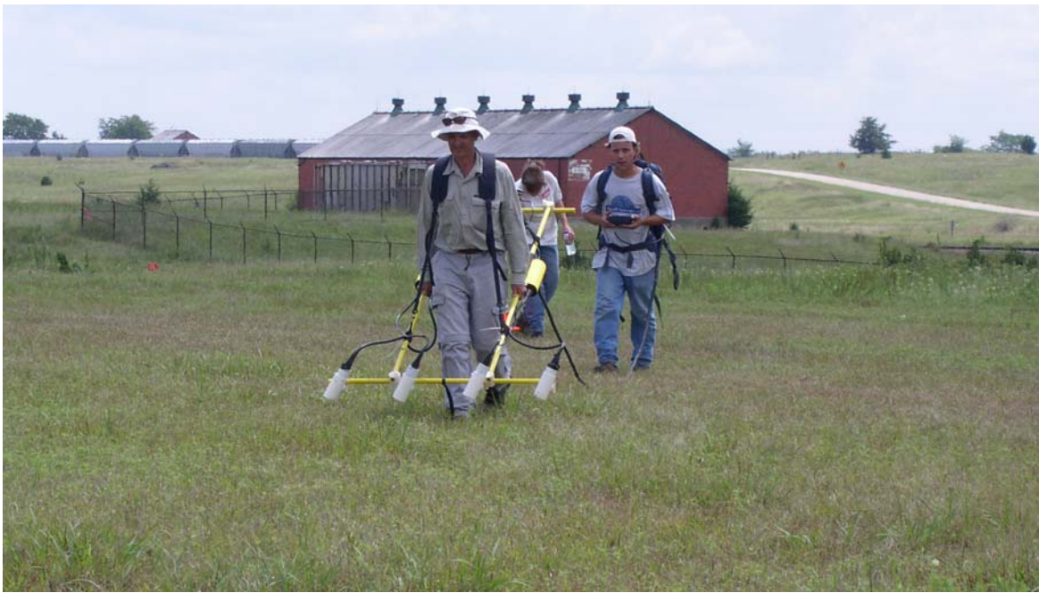
Figure 1. Demonstrator's system, TM-4 MAG array, shown as man portable.
