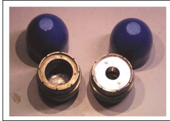
Figure 25. M781BT projectile with actuator mounting.
