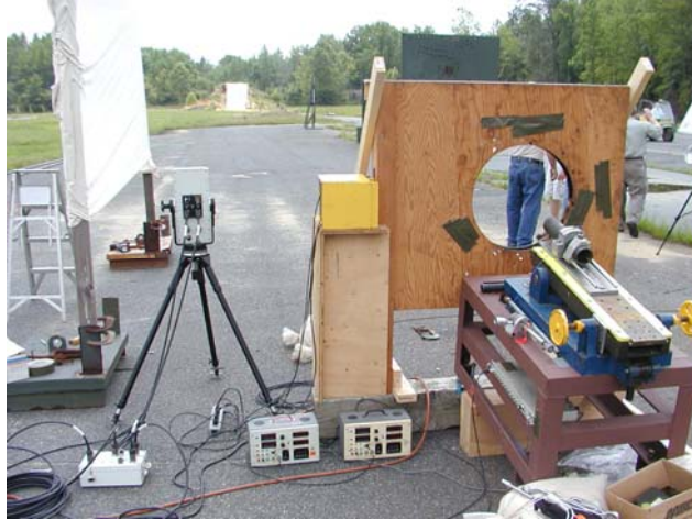
Figure 35. SCORPION open-loop test setup at the ARL Transonic Experimental Facility.
