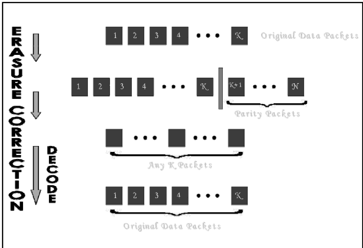
Figure 2.1: Operation of Forward Error Correction (FEC) Method
