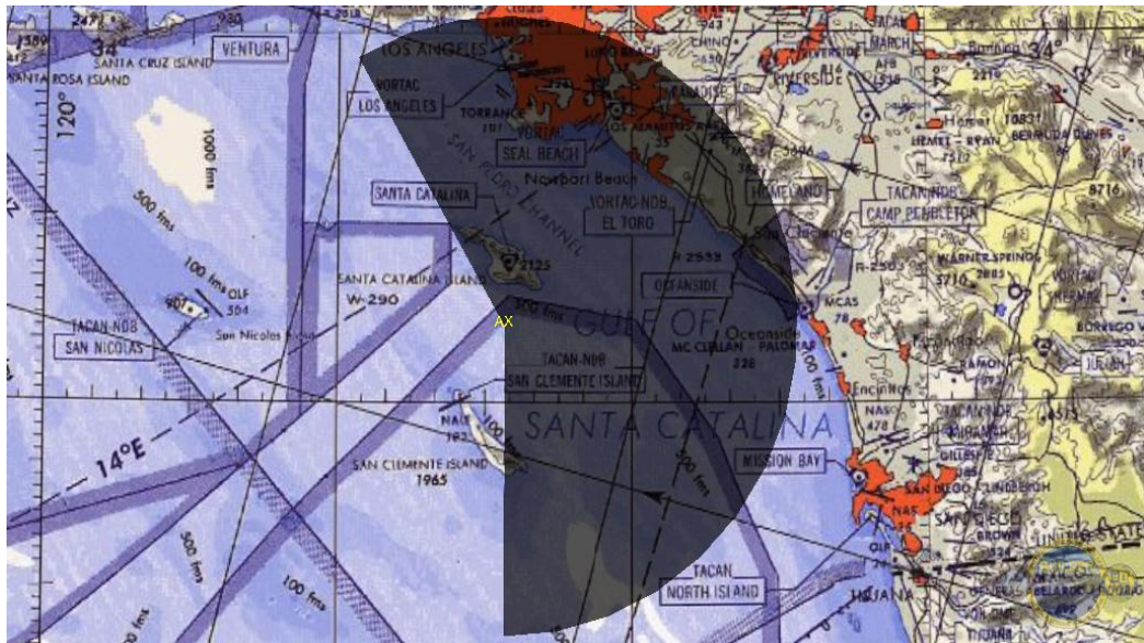
Fig. 28. Builder signal-to-noise ratio plot using the MMWave model for October 8 th at 1933 UTC for 1, 3, 10 and 18 GHz.
