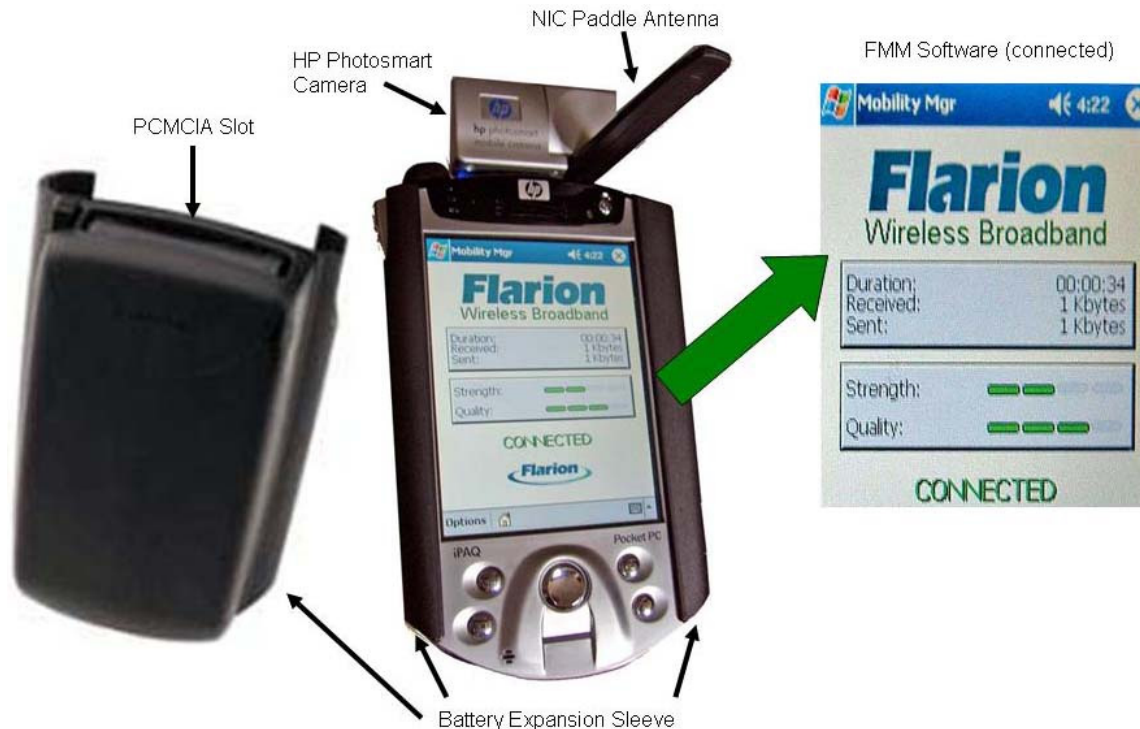
Figure 20. HP iPAQ HX4700 with 802.20 NIC installed in expansion pack running FMM
