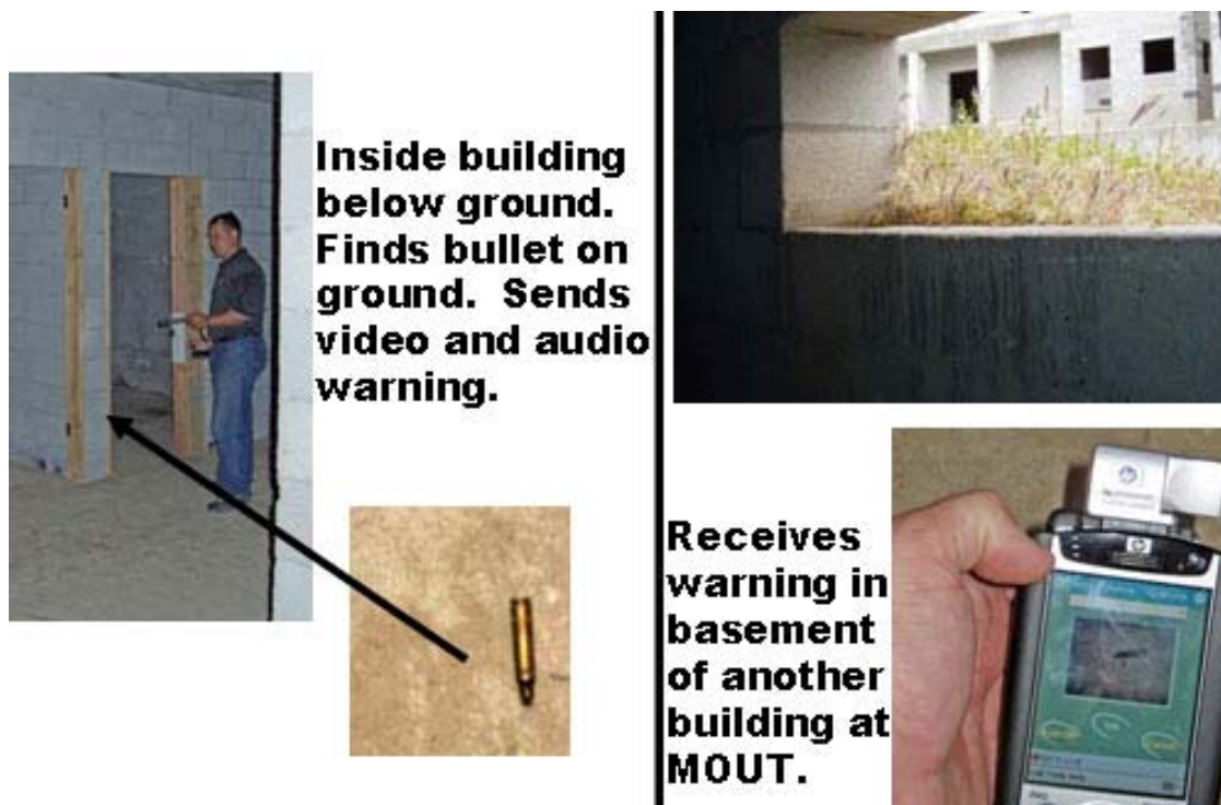
Figure 41. MOUT Early Warning Using Full Duplex Audio and Video
