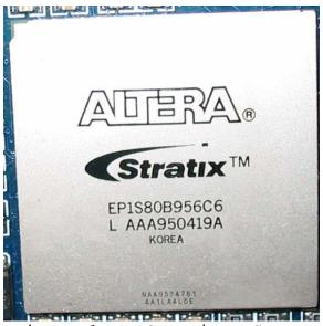
Figure 1. Stratix FPGA.
