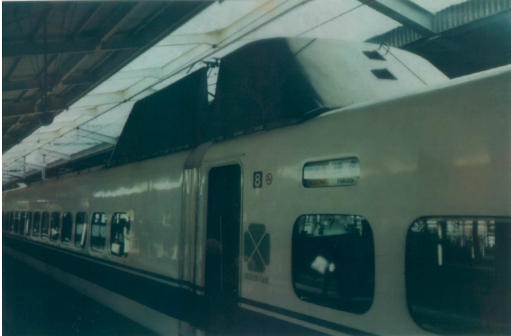
Figure 1. Shroud surrounding a pantograph.
