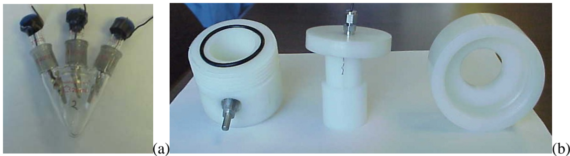
Figure 3: (a) Open and (b) Constrained Fixtures for \text{Mg}/\lambda\text{-MnO}_2 Cell
