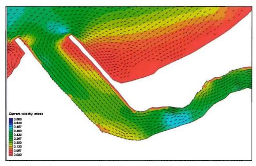
Figure 5-11a. Near-maximum flood-tide velocity, Mattituck Inlet, pre-dredging grid
