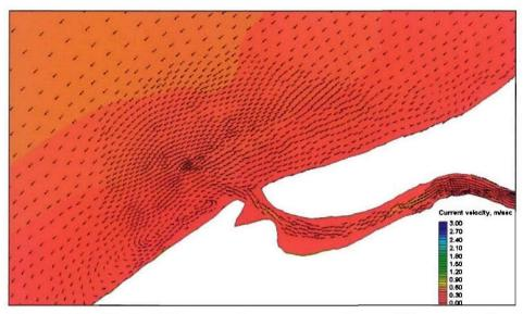
Figure 5-14i. Mattituck Inlet natural state, near maximum offshore spring flood-tide and inlet spring ebb-tide velocity, 0030 on 8 October 2002
