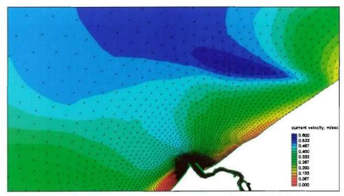
Figure 5-8a. Near-maximum flood-tide velocity, Mattituck Inlet offshore area, 1200 GMT, 7 October 2002
