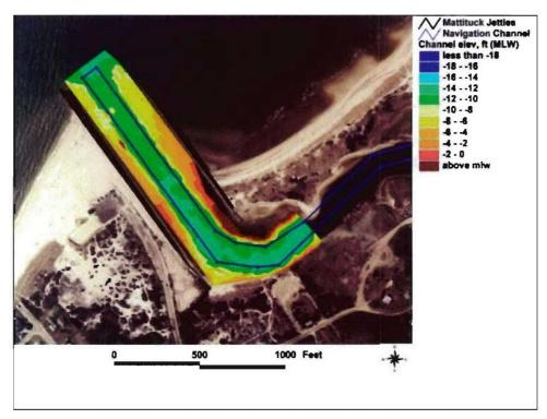
Figure 4-31b. Channel elevation, September 1961 (post-dredging)
