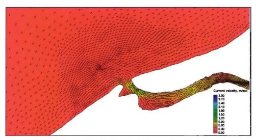
Figure 5-14e. Mattituck Inlet natural state, offshore spring ebb-tide and inlet spring flood-tide velocity, 1530 on 7 October 2002
