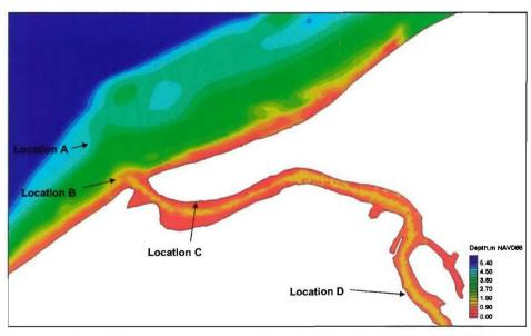
Figure 5-15. Mattituck Inlet assumed (synthetic) natural state and offshore water level and current velocity comparison locations
