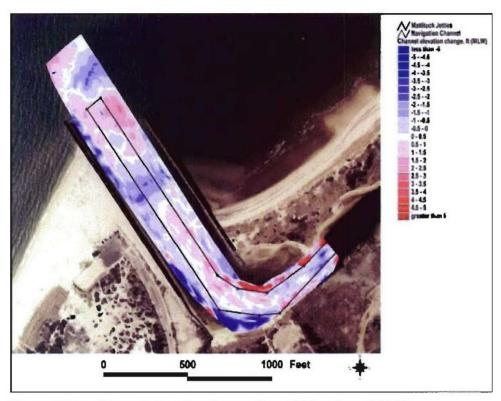
Figure 4-34a. Channel elevation change, May 1980 to August 1983
