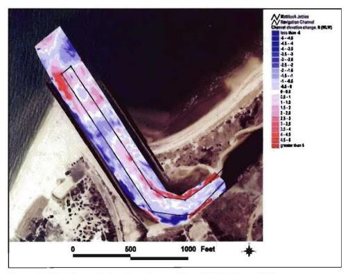
Figure 4-34d. Channel elevation change, May 1980 to June 1988
