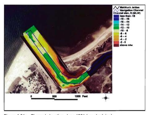
Figure 4-31a. Channel elevation, June 1961 (pre-dredging)
