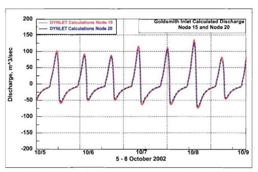
Figure 5-25c. Discharge at Goldsmith Inlet, DYNLET Nodes 15 and 20 calculations, 5-8 October 2002
