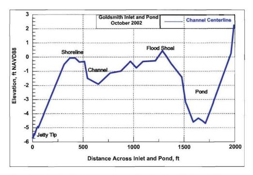
Figure 3-45. Goldsmith Inlet channel center line elevation, 8 October 2002
