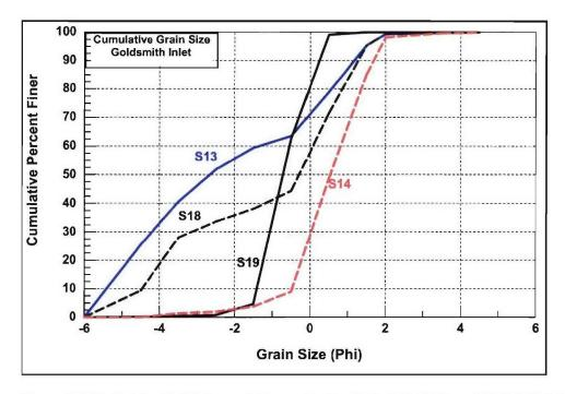
Figure 3-50d. Goldsmith Inlet cumulative grain size S13, S14, S18, and S19, 8 October 2002 and 31 July 2003
