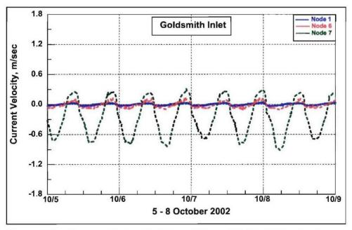
Figure 5-26a. Current velocity calculations offshore of Goldsmith Pond and DYNLET Nodes 6 and 7 calculations, 5-8 October 2002
