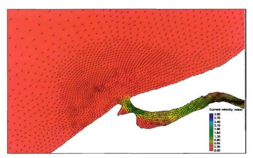
Figure 5-14d. Mattituck Inlet natural state, offshore spring flood-tide and near-maximum inlet spring flood-tide velocity, 1430 on 7 October 2002
