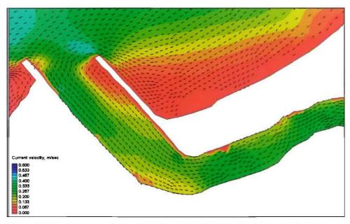
Figure 5-11d. Near-maximum ebb-tide velocity, Mattituck Inlet, post-dredging grid
