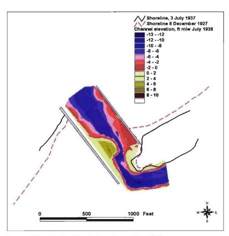
Figure 4-22a. Mattituck Inlet channel elevation, 1938
