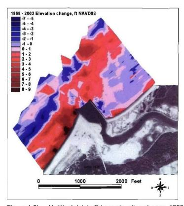
Figure 4-5b. Mattituck Inlet offshore elevation change, 1969-2002
