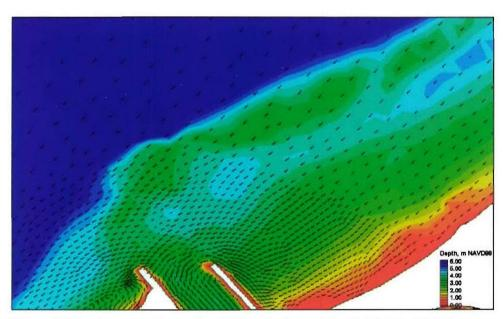
Figure 5-8d. Near-maximum flood-tide velocity and depth, Mattituck Inlet offshore shoal area, 1200 GMT, 7 October 2002
