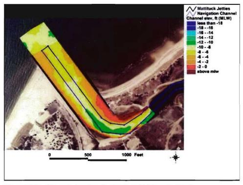
Figure 4-33a. Channel elevation, September 1990 (pre-dredging)
