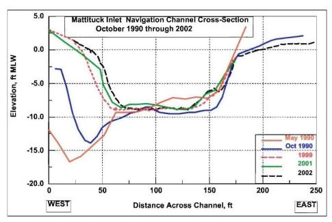
Figure 4-39c. Mattituck Inlet channel cross-section C
