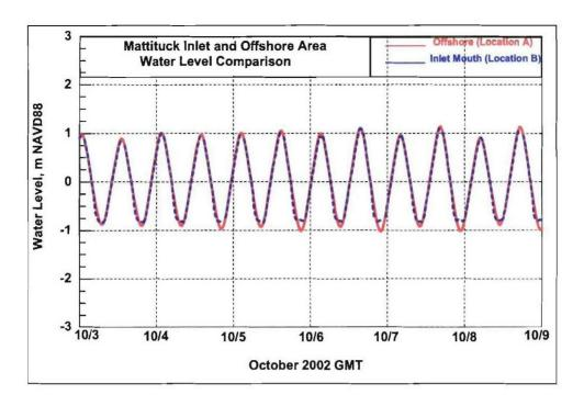
Figure 5-16a. Mattituck Inlet natural state and offshore water level comparison (Locations A and B)
