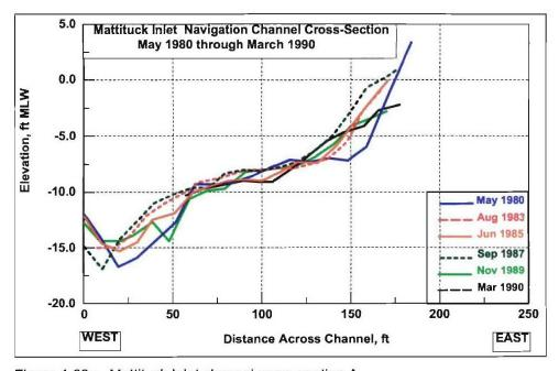
Figure 4-39a. Mattituck Inlet channel cross-section A
