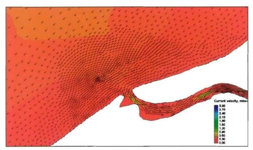
Figure 5-14c. Mattituck Inlet natural state, offshore and inlet spring flood-tide velocity, 1230 on 7 October 2002
