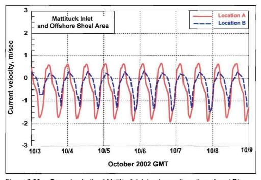
Figure 5-20a. Current velocity at Mattituck Inlet entrance (Locations A and B)
