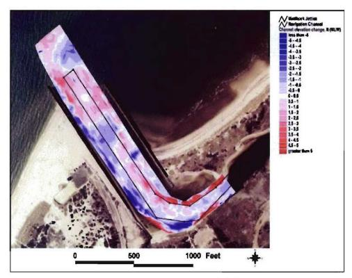
Figure 4-34c. Channel elevation change, May 1980 to September 1987
