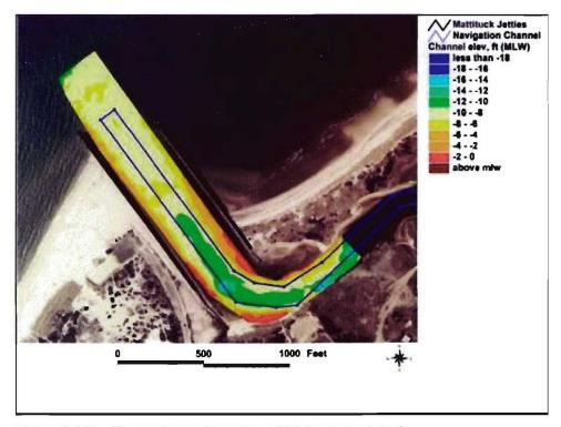
Figure 4-32b. Channel elevation, May 1980 (post-dredging)
