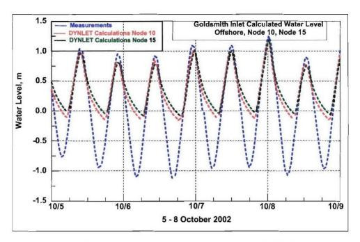
Figure 5-24d. Water-level measurements offshore of Goldsmith Inlet and DYNLET Nodes 10 and 15 calculations, 5-8 October 2002
