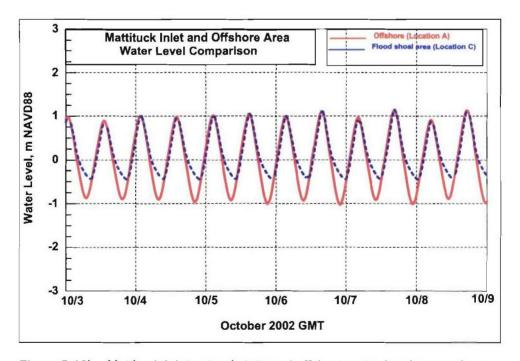
Figure 5-16b. Mattituck Inlet natural state and offshore water level comparison (Locations A and C)
