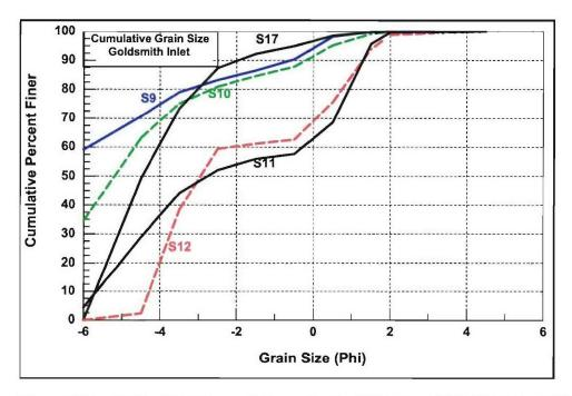
Figure 3-50c. Goldsmith Inlet cumulative grain size S9-S12 and S17, 8 October 2002 and 31 July 2003
