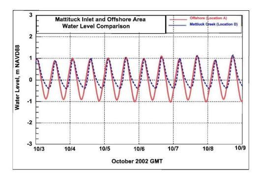
Figure 5-16c. Mattituck Inlet natural state and offshore water level comparison (Locations A and D)
