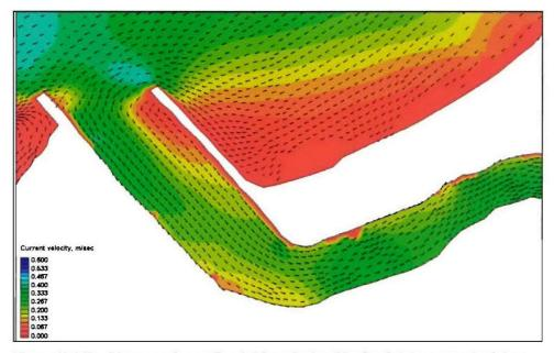
Figure 5-11b. Near-maximum flood-tide velocity, Mattituck Inlet, post-dredging grid
