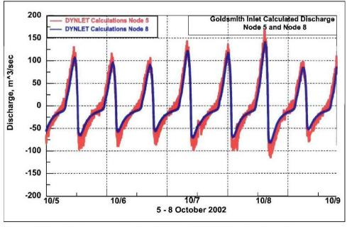
Figure 5-25a. Discharge at Goldsmith Inlet, DYNLET Nodes 5 and 8 calculations, 5-8 October 2002
