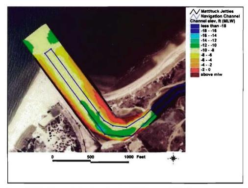
Figure 4-33b. Channel elevation, October 1990 (post-dredging)
