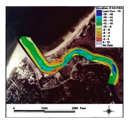
Figure 3-18. Mattituck Inlet Federal navigation channel elevation, 6-8 October 2002
