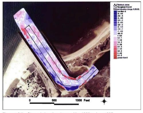
Figure 4-34b. Channel elevation change, May 1980 to June 1985
