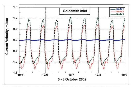
Figure 5-26c. Current velocity calculations offshore of Goldsmith Pond and DYNLET Nodes 8 and 9 calculations, 5-8 October 2002
