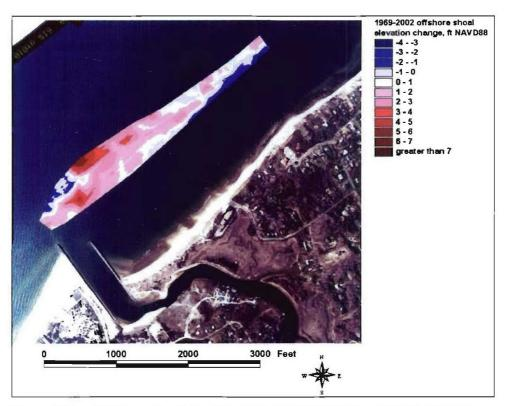
Figure 4-7. Offshore shoal elevation change, 1969-2002 and Mattituck Inlet 16 April 2003
