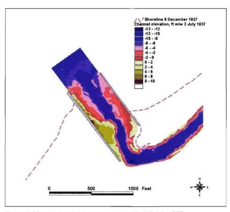
Figure 4-21a. Mattituck Inlet channel elevation, 3 July 1937
