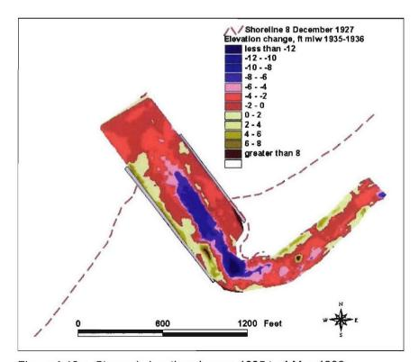
Figure 4-19c. Channel elevation change, 1935 to 4 May 1936
