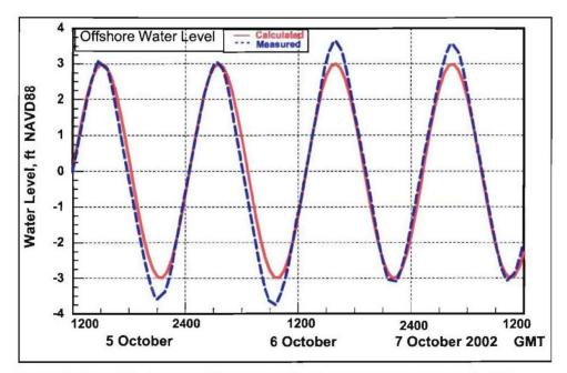
Figure 6-3. Mattituck Inlet offshore water-level measurements and calculations by CEA model
