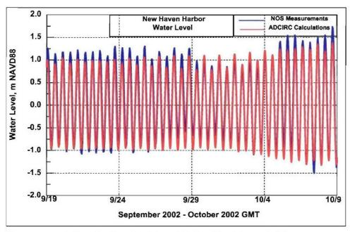
Figure 5-5c. Water level at New Haven Harbor, New Haven; NOS measurements and ADCIRC calculations, 19 September - 8 October 2002
