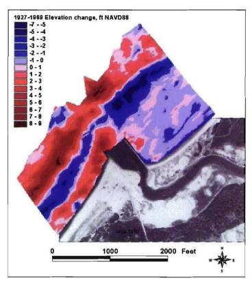
Figure 4-5a. Mattituck Inlet offshore elevation change, 1927-1969
