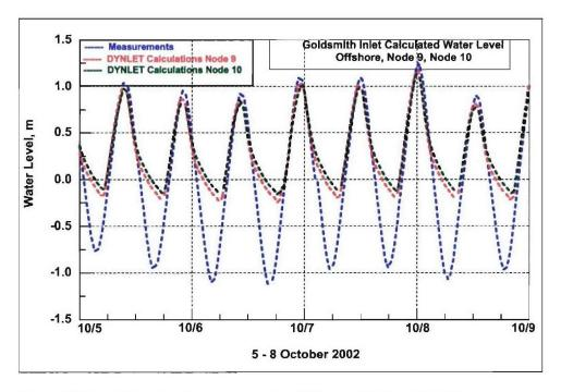
Figure 5-24c. Water-level measurements offshore of Goldsmith Inlet and DYNLET Nodes 9 and 10 calculations, 5-8 October 2002
