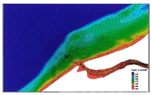
Figure 5-18h. Near-maximum inlet ebb-tide velocity and depth, Mattituck Inlet offshore shoal area, 2030 GMT on 7 October 2002
