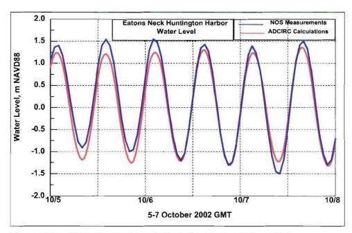
Figure 5-5b. Water level at Eaton's Neck, Huntington Harbor; NOS measurements and ADCIRC calculations, 5-8 October 2002
