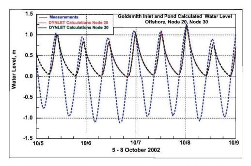
Figure 5-24f. Water-level measurements offshore of Goldsmith Inlet and DYNLET Nodes 20 and 30 calculations, 5-8 October 2002
