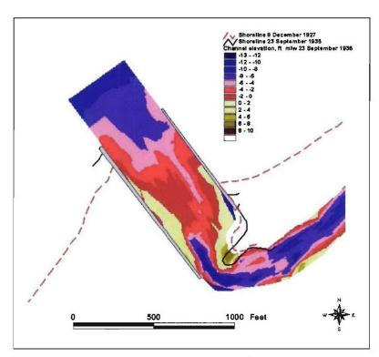
Figure 4-18a. Mattituck Inlet channel elevation, 1935
