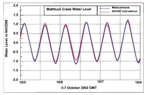
Figure 5-6d. Water level at Mattituck Creek; measurements and ADCIRC calculations, 5-7 October 2002
