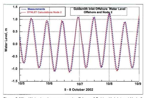
Figure 5-22b. Water-level measurements offshore of Goldsmith Inlet and Node 2 calculations, 5-8 October 2002
