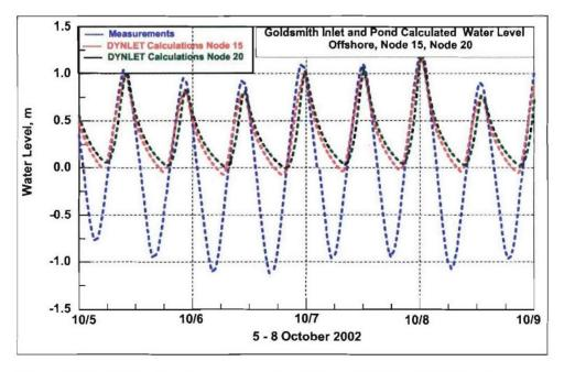
Figure 5-24e. Water-level measurements offshore of Goldsmith Inlet and DYNLET Nodes 15 and 20 calculations, 5-8 October 2002
