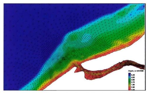
Figure 5-18d. Near-maximum inlet flood-tide velocity and depth, Mattituck Inlet offshore shoal area, 1430 GMT on 7 October
