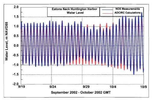
Figure 5-5a. Water level at Eaton's Neck, Huntington Harbor; NOS measurements and ADCIRC calculations, 19 September - 8 October 2002
