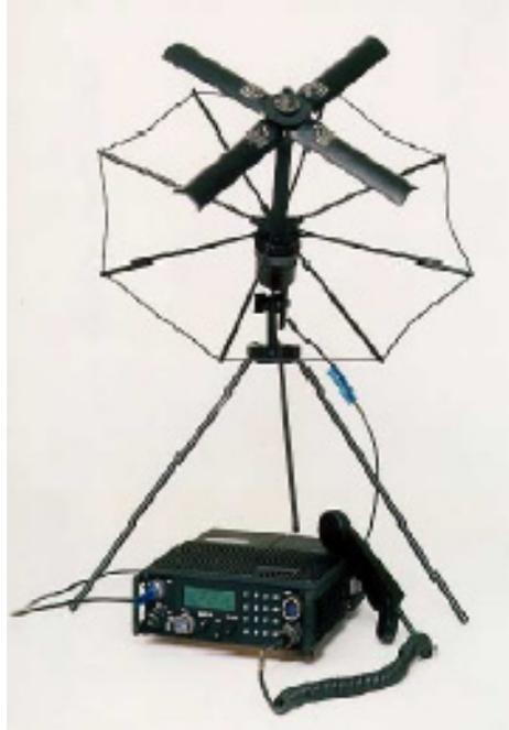
Figure 36. AN/PSC-5 Tactical Satellite Telephone/Radio [From Ref 19]
