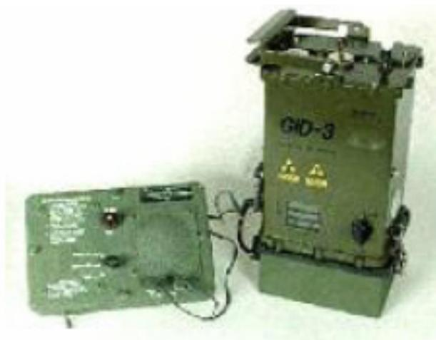
Figure 39. Chemical Sensor [From Ref 19]
