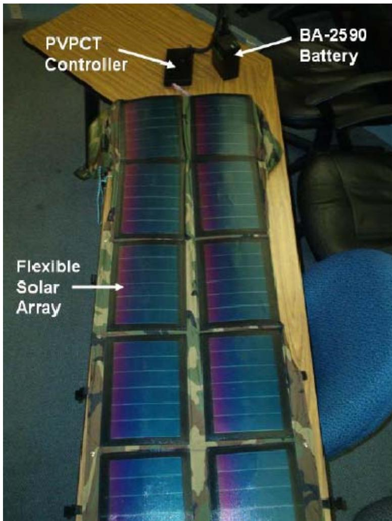
Figure 45. PVPCT System Prototype With Flexible Solar Array Deployed [From Ref 20]
