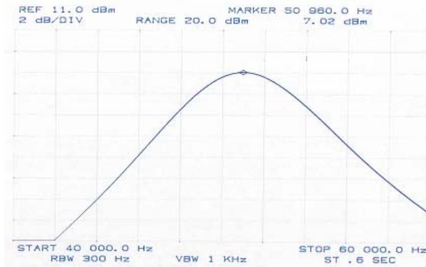
Figure 53. Actual Frequency Response: Center Frequency = 50.560 kHz,  $Q_p = 9.711$
