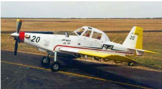
Figure 9. Air Tractor AT-802, Crop Duster Version (Jane's)
